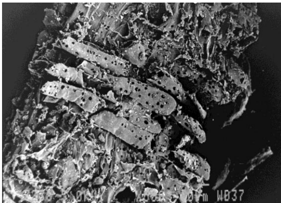
Fig: 11(b). SEM image of activated sawdust
